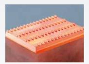
An electrode with 64 pins for core plate is processed by the UH430L.
