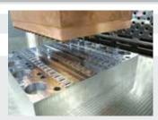
Corner edges of apertures are finished by the AP3L, the super-high precision sink EDM using the electrode which has been made in process step 4.
