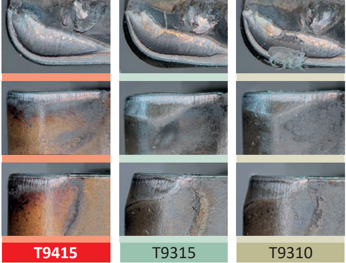
Photos from continuous cutting. All taken after 16 minutes.
